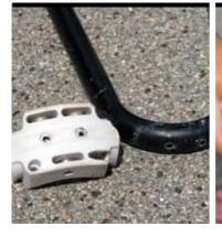
Remove the old cleat by drilling through the blind rivets. If they start to spin, show them no mercy – use a screwdriver or awl to remove them.
