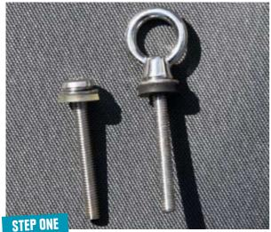
Cut the bolts so that the effective length is the same as the original. Both washers (stainless and rubber) need to be roughly the same size. The bolts may already come with washers (as in picture 2), but bigger washers are needed to spread the load, and the rubber washers are for spreading it evenly.
