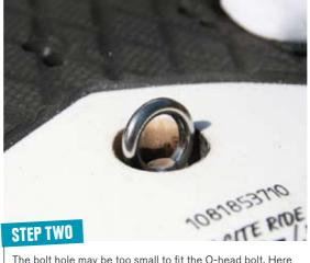
The bolt hole may be too small to fit the O-head bolt. Here I needed to file off just a little bit of the edge. Make sure that you put some Loctite glue over the exposed material to protect it from water.
